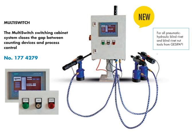
The device enables monitoring of the minimum setting force and the number of connectors set. This system can be realised with any pneumatic hydraulic GESIPA® setting tool. It is irrelevant whether blind rivets, blind rivet nuts or a combination of various connectors are being processed here.
