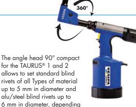
on the tool Type. The minimum edge clearance is 12 mm, the head length is 90 mm. Both angle heads can be freely fixed in any position aroand the TAURUS<sup>®</sup> tensile axis (360° free rotation).
