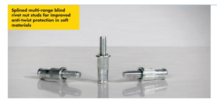
The new GESIPA® splined PolyGrip® blind rivet nut studs made from M6 and M8 steel are a further development of the well-proven PolyGrip® multi-range blind rivet nuts. They combine the advantages of covering large grip ranges with the knurling for increased anti-twist protection. The long longitudinal knurling ensures uniform setting characteristics over the entire grip range and a large closing head.
