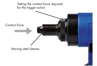
This feature ensures that the materials of the riveting application will be pressed together before the rivet is installed, thus avoiding gaps in between. Moreover the operator will be certain that the rivet has reached its end position in the application and that the setting head is in contact with the upper side of the material. The pressing force can be adjusted variably with springs depending on the application.
