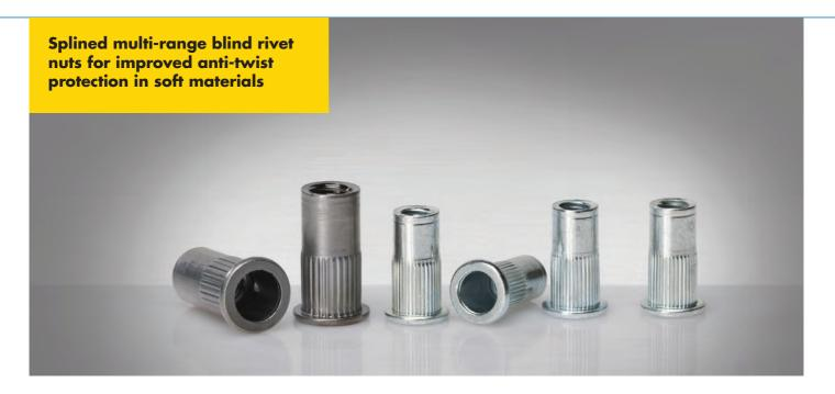
The new GESIPA® splined PolyGrip® blind rivet nuts made from M6 and M8 steel are a further development of the well-proven PolyGrip® multi-range blind rivet nuts. They combine the advantages of covering large grip ranges with the knurling for increased anti-twist protection. The long longitudinal knurling ensures uniform setting characteristics over the entire grip range and a large closing head.
