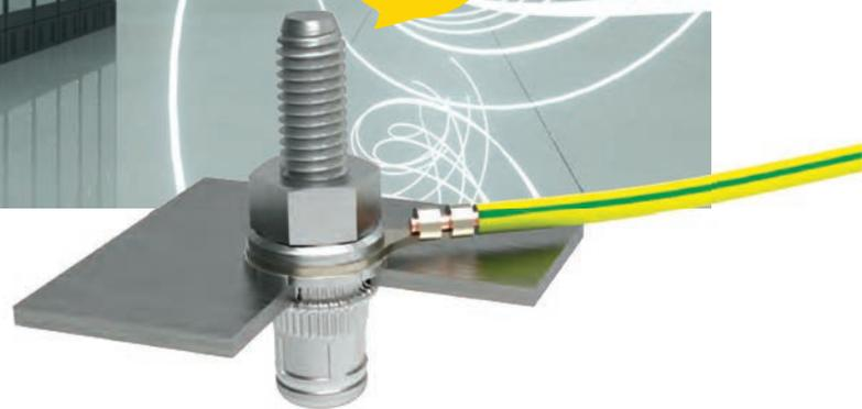
The GESIPA® blind rivet nut stud for earthing and protective conductor connections offers a high degree of flexibility and quick installation of a protective conductor connection when mounted in a control cabinet.
