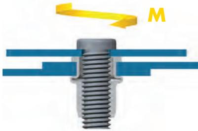
The thread must still turn smoothly in order to pass the test. Then the blind rivet nut is loaded again up to the overtorque.
