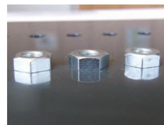
Inserted nut after process has been finished.
