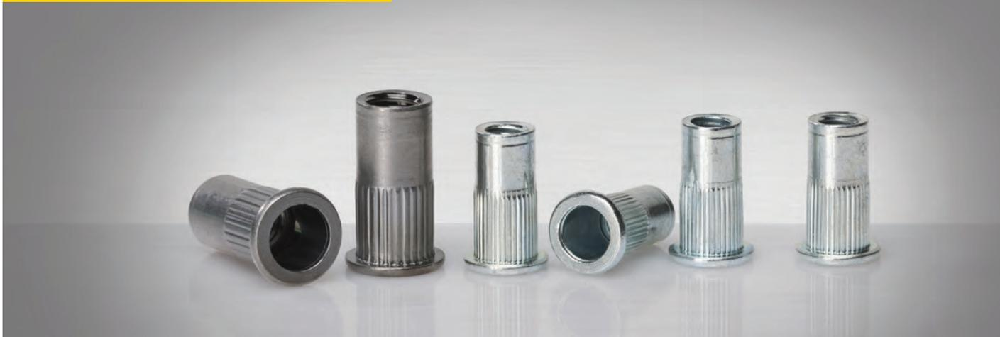
The new GESIPA® splined PolyGrip® blind rivet nuts made from M6 and M8 steel are a further development of the well-proven PolyGrip® multi-range blind rivet nuts. They combine the advantages of covering large grip ranges with the knurling for increased anti-twist protection.
