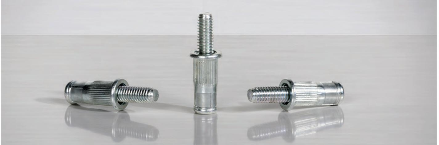
The new GESIPA® splined PolyGrip® blind rivet nut studs made from M6 and M8 steel are a further development of the well-proven PolyGrip® multi-range blind rivet nuts. They combine the advantages of covering large grip ranges with the knurling for increased anti-twist protection.
